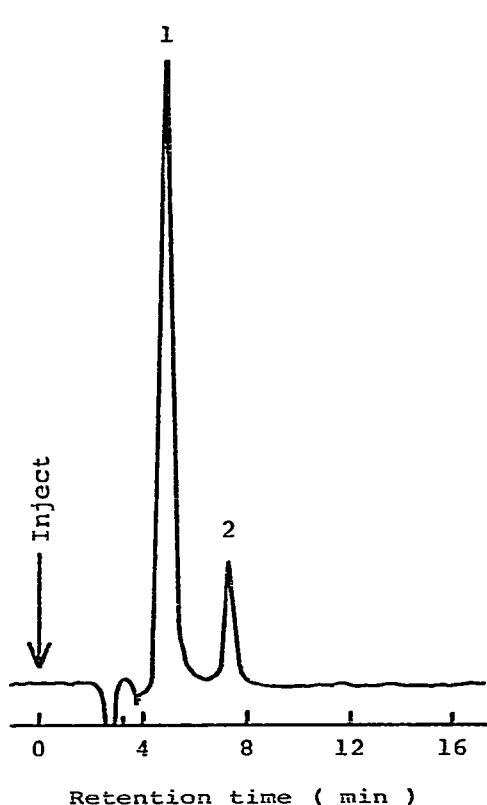
Fig. 6. Chromatogram of waste water. Sample size, 10 \mu l. Peaks: 1 = \text{Cl}^- (200 nmol); 2 = \text{SO}_4^{2-} (15 nmol).
